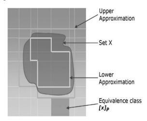
Using the features in the set P through equivalence Class we can construct Upper and Lower Approximations.
